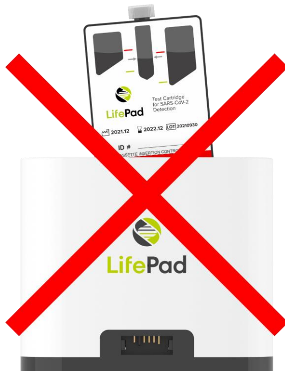
Picture 29. Test Cartridge Incorrect Positioning
