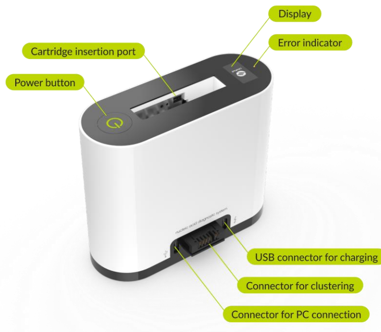
Picture 2. Main Controls Location
